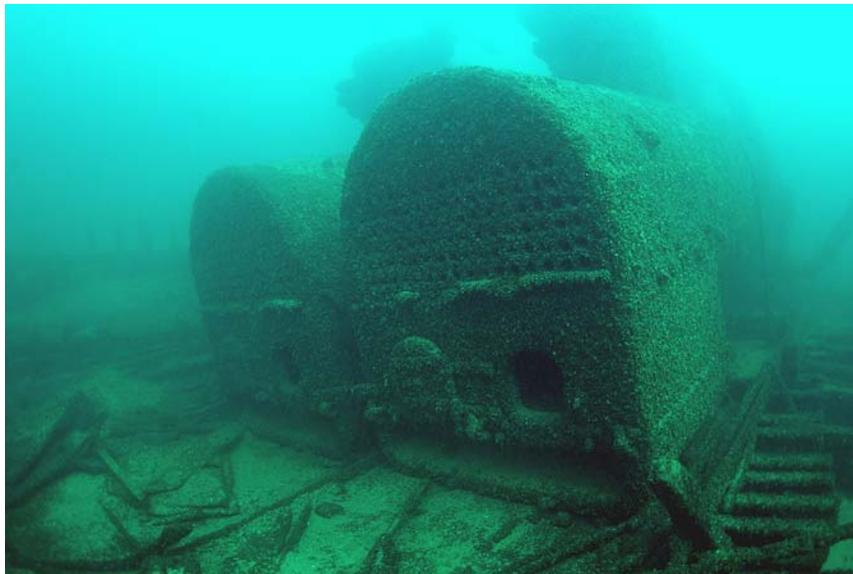
Figure 72. The *Selah Chamberlain*'s twin boilers are still attached to the steple compound engine. Tamara Thomsen.
